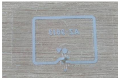
Etiqueta B - WET INLAY UHF H3 96/512B 12x9 mm
